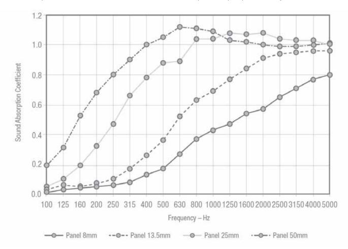
The sound absorption has been tested in accordance with AS/ISO 354. For complete test reports please contact your local distributor.
