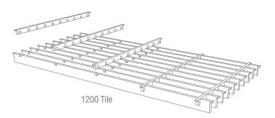
**Step 1**Remove components from packaging and assemble the profiles together, paying attention to the junctions of each profile as they fit tightly within each other.
