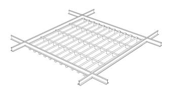
**Step 3**Manouvre the ceiling tile above the ceiling grid supports and place directly on T bar sections as shown. Ensure ceiling tile is centred.
