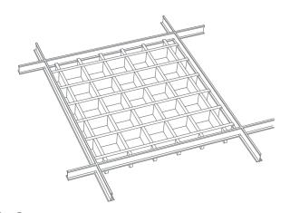
**Step 3**Manouvre the ceiling tile above the ceiling grid supports and place directly on T bar sections as shown. Ensure ceiling tile is centred.
