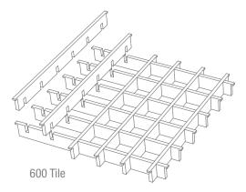
**Step 1**Remove components from packaging and assemble the profiles together paying attention to the junctions of each profile as they fit tightly within each other.
