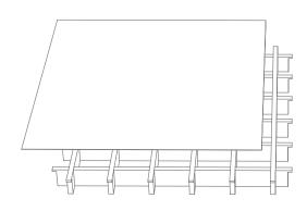
**Step 2**Place the Infill on the back of the tile.
