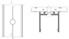
Secure appropriate fasteners into substrate through pre-drilled holes in baffle extrusion.
