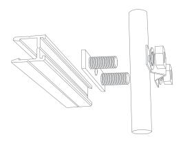
Slide collar and rail along extrusions, and baffle assembly along rods to desired location if necessary. Tighten nuts over collar to lock baffle in position.
