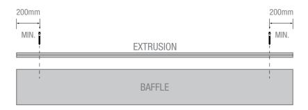
Suspension points should be placed minimum 200mm from either end of the baffle.
