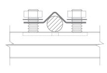
Place collars over rods and mounting studs, screw hand tighten nuts and washers over mounting studs.
