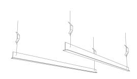
Install 'tee' bars to manufacturer's specification at desired level. Minimum two 'tee' bars per baffle span.
