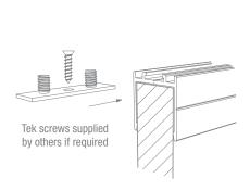
After extrusion is secured to baffle, insert sliding rails into extrusion.
