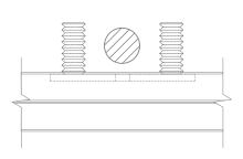
Offer baffle assembly to structural rods ensuring rods are centred between mounting studs. (Minimum 2 rods per baffle span).
