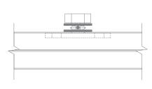
Hand tighten nuts over assembly, capturing the cable between the washers.
