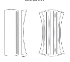
Follow the same procedure above for column installations of baffle.
