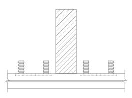
Offer baffle assembly to building structure ensuring it is centred between two sliding rails. (Minimum 2 structural components per baffle span).
