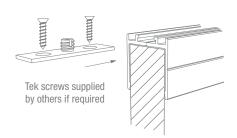
After extrusion is secured to baffle, insert sliding rails into extrusion.
