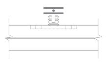
Offer baffle assembly to structural cables ensuring cables are centred within fastener cavity and between washers.
