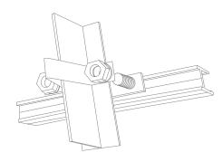
Slide collar and rail along extrusions, and baffle assembly along 'tee' bar to desired location if necessary. Tighten nuts over collar to lock baffle in position.
