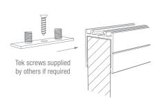
After extrusion is secured to baffle, insert sliding rails into extrusion.
