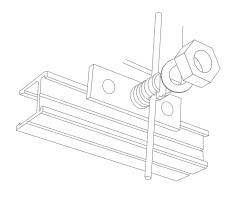
Slide rails along extrusions, and baffle assembly along cables to desired location if necessary. Tighten nuts over washers to lock baffle in position.
