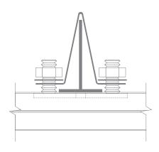
Place collars over 'tee' bars and mounting studs. Screw hand tighten nuts and washer over mounting studs.
