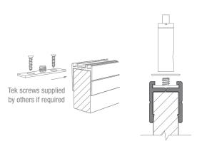
After extrusion is secured to baffle, insert sliding rail into extrusion. Secure cable fixture to exposed screw head with supplied washer between.
