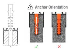
Attach extrusion to baffle and reverse-drill hole for anchor into baffle through pre-drilled holes in extrusion.\* Insert the anchor into baffle.
