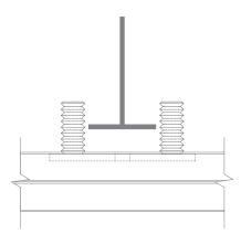
Offer baffle assembly to ceiling 'tee' bar ensuring 'tee' bars are centred between mounting studs.
