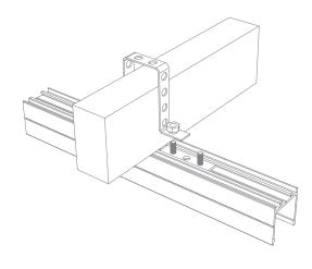
Slide strap and rails along extrusions, and baffle assembly along structural components to desired location if necessary.
