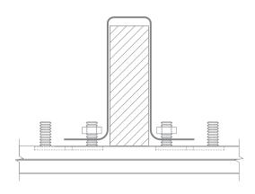
Measure and cut strap to length, place strap over structural components and mounting studs, screw hand tighten nuts and washers over mounting studs.
