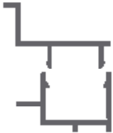
Frame Base + Frame Capping Essential and sold separately Supplied in 2750mm lengths
